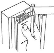
\*\*The 1" Panel must be snapped into the frame Fixing strip FIRST.
