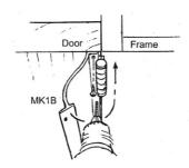
Butt L shaped edge to the door side of hinges while aligning with top and bottom of door. Secure completely with TEK self tapping screws
