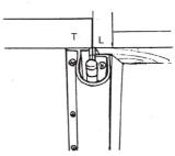
Architrave frame fitted with MK1B reversed, due to limited space on the frame side
