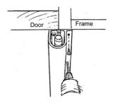
Roll the MK1B over the hinges and butt the T shape to hinges on frame side. Align with L shape top and bottom. Secure with TEK self tapping screws and remove cellophane protective membrane. You are now fingersafe
