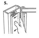
Place the 1" panel next to the gripper of the frame fixing strip. Align top and snap into place.
