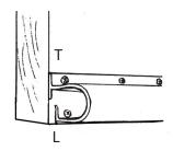
Roll ToeSafe up and align T shape to meet L shape top and bottom. Expose adhesive strip and secure on door. Secure completely using TEK self tapping screws provided.
