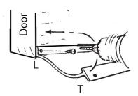
Align L shaped edge to the bottom of door. Hold components in position and expose adhesive. Secure with screws provided.
